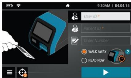
2. Input the Patient ID and/or Order # using the integrated barcode scanner or manually enter the data using the on-screen key pad.
