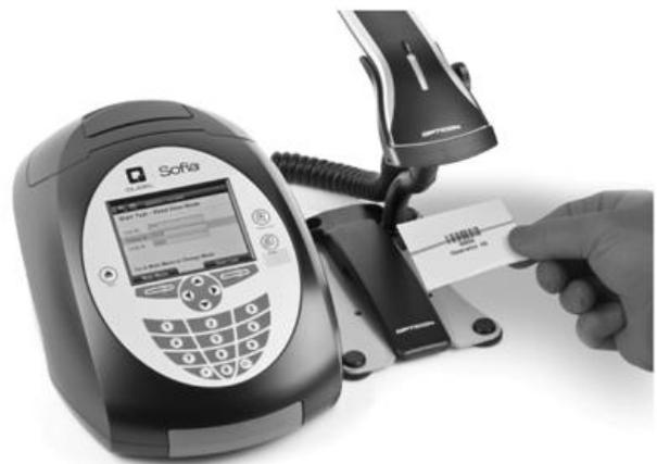
3. Input Patient ID or Order # using the barcode scanner or manually enter the data using the key pad.
