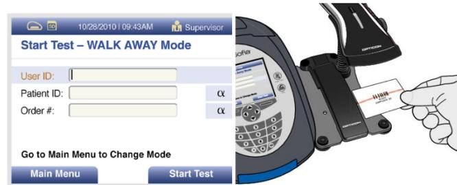
2. Input the Patient ID and/or Order # using the handheld barcode scanner or manually enter the data using the key pad.
