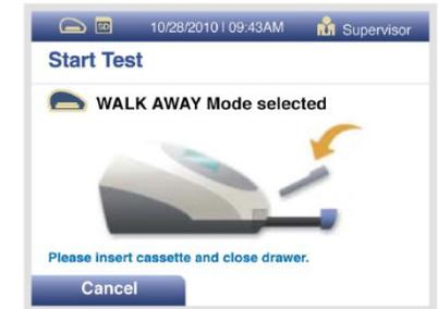
4. Verify that the correct mode, WALK AWAY or READ NOW, has been selected. Insert the Test Cassette into the drawer. Then gently close the door.
